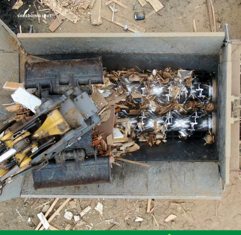
The shredding drums are effectively protected against wear by armouring in exposed zones.
